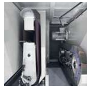
__ deburring and edge rounding with an abrasive contact roller and cross belt system
