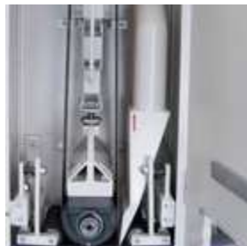
__ FC120 Z has one abrasive belt unit
