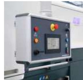
___ possibility of regulating which stations will work and at what speed, the working pressure for both stations, floating drum on/off and drum oscillation
