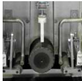
__ abrasive belt head surface finishing and imperfections removal for rectangular tubes and flat bars
