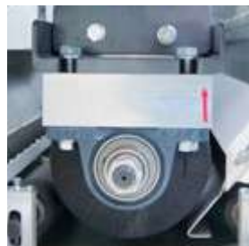
___ brush unit with option to be used with oscillation (150 strokes/min)
