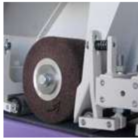
__ smooth finishing after belt grinding operation with non-woven brush
