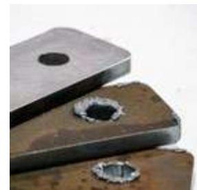
___ smooth edges two cross belts mounted with abrasive blocks running in opposite directions
