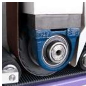
__ abrasive belt head surface finishing and imperfections removal for square and rectangular tubes, flat bars and small sheet metal
